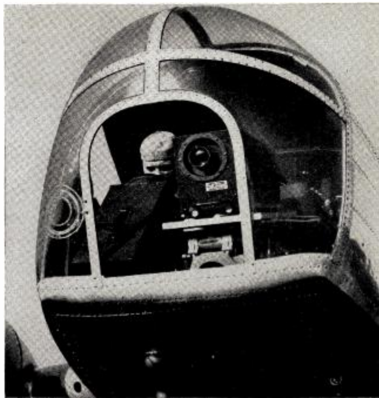
Mounted in the nose of an airplane, special RCA airborne television equipment will give ground observers a sharp, clear, bird's-eye view of land and sea.
